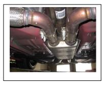
1. To remove your stock exhaust, unbolt it from the clamps located just after the manifolds then remove the whole exhaust system
