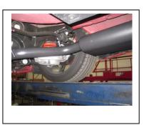
3. Now install the passenger side tailpipe assembly #B by sliding the metal hangers into the rubber grommets. Use clamp #D to secure together.
