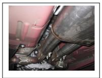
2. Install your Gibson muffler Assembly
