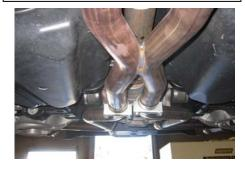
6. Use stainless steel cleaner to prevent tip from discoloration. Inspect all fasteners after 25-50 miles of operation and re-Tighten as necessary
