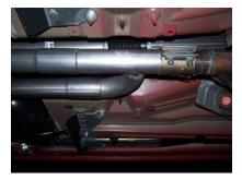
7. After kit is installed, adjust your kit so it does not hit or rub on anything. Check that your exhaust tips are not touching your bumper. After checking everything, now tighten all clamps starting from the front and working your way to the rear. Use stainless steel cleaner and a Scotch Brite pad weekly to prevent tip from discoloration. Inspect all fasteners after 25-50 miles of operation and re-tighten as necessary.
