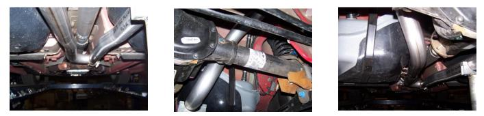
6. Install h-pipe adapter onto tailpipes. Use your factory clamp to attach it to your stock pipe. Do not tighten. Use clamps #D to attach your adapter to your tail pipe. Do not tighten.
