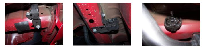
4. Now you are going to install the system in reverse order. First, install your new Gibson mufflers. There are specific left and right assemblies. Install rear muffler hangers using bolts from rubber grommet hanger. They are self-tapping bolts.
