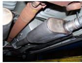
4. Install mufflers #C onto head pipes 11/2"-2" with the louvers facing towards the converter. Use a jack stand to support the muffler. Use clamps #I to secure the muffler to the headpipe. DO NOT TIGHTEN. Muffler inlet is looking into the louvers.
