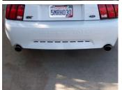
down securely. Use stainless steel cleaner and a Scotch Brite pad weekly to prevent tip from discoloration. Inspect all fasteners after 25-50 miles of operation and retighten as necessary.
