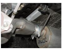
INSTALL FRONT MUFFLER HANGER #F INTO RUBBER GROMMETS LOCATED JUST ABOVE THE INLET OF THE MUFFLER. USE THIS CLAMP TO SECURE HEADPIPE. DO NOT TIGHTEN.
