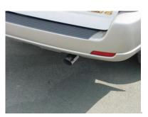
INSTALL THE STAINLESS TIP #E. TO CLEAN TIP USE ANY STAINLESS OR ALUMINUM CLEANER AND A SCOTCH BRITE PAD. NOW GO BACK AND TIGHTEN ALL NUTS, BOLTS AND CLAMPS STARTING FROM THE FRONT AND WORKING BACK.
