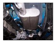
**3.** Install muffler #B onto head pipe  $1\frac{1}{2}$ "-2" with the louvers facing towards the converter. Use a jack stand to support the muffler. Use clamp #F to secure the muffler to the headpipe. DO NOT TIGHTEN.
