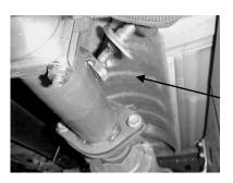
LAY OUT THE GIBSON EXHAUST ON THE FLOOR AND COMPARE PART NUMBERS WITH THE MANUAL. REMOVE THE FACTORY O2 SENSOR LOCATED IN FRONT OF THE MUFFLER.YOU WILL RE-USE YOUR FACTORY O2 SENSOR GASKET. THEN CUT STOCK EXHAUST DIRECTLY BEHIND THE MUFFLER. USE WD-40 ON ALL RUBBER GROMMETS, NUTS AND BOLTS FOR EASY REMOVAL.
