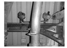
INSTALL HANGER #DINTO THE REAR MUFFLER RUBBER GROMMETS. THE VERTICAL RODS WILL BE FACING TOWARDS THE REAR OF THE TRUCK.
