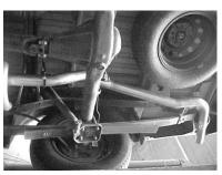
SLIP THE OVER AXLE PIPE #C INTO THE OUTLET OF THE MUFFLER NO MORE THEN 2" AND NO LESS THEN 1". USE CLAMP # E TO SECURE TAILPIPE TO MUFFLER. DO NOT TIGHTEN. INSERT WELDED HANGER INTO RUBBER GROMMET.
