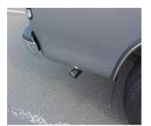
NOW INSTALL THE STAINLESS STEEL TIP USE ANY ALUMINUM OR STAINLESS STEEL CLEANER TO POLISH YOUR TIP. TIGHTEN ALL CLAMPS AND HANGERS STARTING FROM THE HEADPIPE BACK
