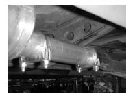
Install head pipe # A 1" to 1  $\frac{1}{2}$ " on to your existing stock front pipe and secure with clamp # G. Do not tighten.
