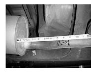
Lay out the exhaust on the floor so it looks like the drawing and compare parts with manual. To remove the stock exhaust cut 8 1/2" inches in front of the muffler. Leave all rubber grommets in place. Use WD-40 to aid in removal of exhaust and hangers.
