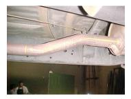
Lay out the exhaust on the floor so it looks like the drawing and compare parts with manual. **To remove the stock exhaust Cut it 17 1/2" in front of the muffler.** Leave all rubber grommets in place. Use WD-40 to aid in removal of exhaust and hangers.
