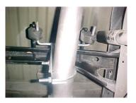
Next install rear muffler hanger # D into grommets at just about the outlet of the muffler clamp onto tailpipe. Do not tighten.
