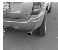
INSTALL YOUR STAINLESS STEEL TIP. USE ANY ALUMINUM OR STAINLESS STEEL CLEANER TO POLISH YOUR TIP. CHECK ALL YOUR CLEARANCES AND TIGHTEN ALL CLAMPS AND HANGERS.
