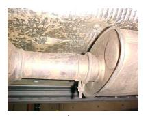
/ UNCLAMP FOR EASIER REMOVAL OF THE FACTORY EXHAUST. CUT THE TAILPIPE BEHIND THE MUFFLER. THEN REMOVE THE FACTORY MUFFLER AT THE CLAMP IN FRONT OF THE MUFFLER. USE A JACK STAND TO SUPPORT THE CONVERTER ONCE EXHAUST IS REMOVED. NOTE LEAVE ALL FACTORY RUBBER GROMMETS IN PLACE
