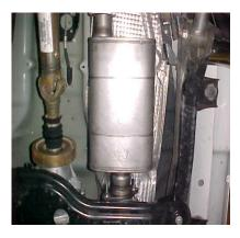
LAY OUT THE GIBSON EXHAUST ON THE FLOOR SO IT LOOKS LIKE THE DRAWING AND COMPARE IT TO THE MANUAL. TO REMOVE THE STOCK **FXHAUST CUT OFF** TAILPIPE JUST BEHIND THE MUFFLER THEN REMOVE MUFFLER FROM 2- BOLT FLANGE JUST IN FRONT OF MUFFLER, LEAVE ALL RUBBER GROMMETS IN PLACE. USE WD-40 TO AID IN REMOVAL OF EXHAUST AND HANGERS.
