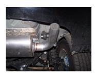
7. Slide exit pipe #E into muffler 1.5-2". Insert welded hanger into rubber grommet. Secure with clamp #G. Do not tighten.
