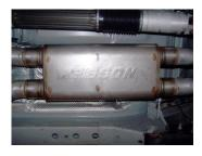
4. Install muffler #C onto headpipes 1.5-2". Use a jack stand to support muffler. Use clamp #G to attach muffler to headpipes. Do not tighten.
