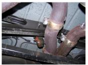
exhaust, unbolt the tailpipes at the clamps behind the over axle pipe. Then disengage hangers from the rubber grommets, and remove the rear tailpipes and mufflers. Now remove all other hangers from rubber grommets and unbolt the rest of the exhaust system at the 2 flanges in front of the stock muffler.
