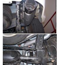
Install the over axle tail pipe w/welded resonator onto extension pipe, insert welded hangers into grommets and use clamp #E to secure pipes together. DO NOT TIGHTEN.
