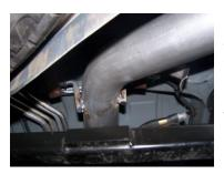
Install extension pipe #C into the muffler  $1\frac{1}{2}$ -2". Insert welded hanger into rubber grommet. Secure the muffler using clamp #E. DO NOT TIGHTEN.
