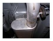
**4.** Install extension pipe #C into the muffler  $1\frac{1}{2}$ -2". Insert welded hanger into rubber grommet. Secure to muffler with clamp #F. DO NOT TIGHTEN.
