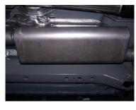
Install muffler #B onto head pipe #A  $1\frac{1}{2}$ -2" with the louvers facing towards the converter. Use a jack stand to support the muffler. Use clamp #F to secure the muffler to the head pipe. DO NOT TIGHTEN. Muffler inlet is looking into the louvers.
