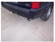
Install stainless steel tip. Clamp down. When you have everything in place, firmly tighten all bolts and clamps down securely. To clean stainless steel tips, use stainless steel cleaner and a Scotch Brite pad.
