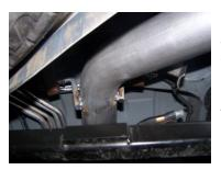
Install extension pipe #C into the muffler 1½-2". Insert welded hanger into rubber grommet. Secure the muffler using clamp #F. DO NOT TIGHTEN.
