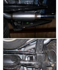
Install the over axle tail pipe w/welded resonator onto extension pipe, insert welded hangers into grommets and use clamp #F to secure pipes together. DO NOT TIGHTEN.
