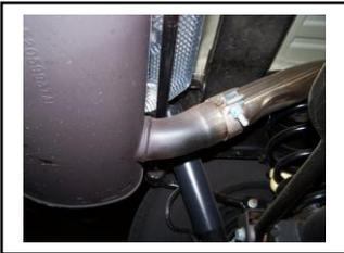
**2.** To remove the stock exhaust, unbolt band clamp located just behind your factory muffler. Disengage the welded hangers using WD-40 from the OEM rubber grommets. Do not damage or remove the rubber grommets as you will reuse them to mount your new system.
