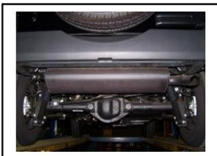
**4.** Install muffer onto head pipe #A 1½"-2" with the louvers facing towards the inlet. Use a jack stand to support the muffer. Use clamp#E to secure the muffer to the headpipe. Do not tighten. Muffer inlet is looking into the louvers.
