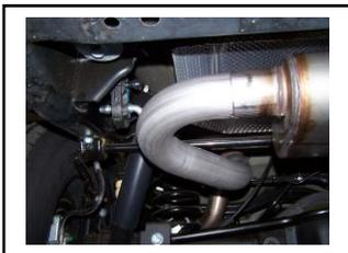
**3.** Install head pipe #A onto your existing stock front pipe and attach with clamp #E. Insert welded hanger into rubber grommet. Do not tighten.
