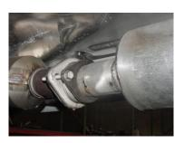
INSTALL FLANGE #B ONTO THE HEADPIPE #A. USE BOLT KIT #G TO SECURE HEADPIPE #A TO STOCK FLANGE. DO NOT TIGHTEN.
