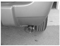
6.) NEXT, INSTALL YOUR STAINLESS STEEL TIP TO YOUR DESIRED LOOK. TO **CLEAN THE** STAINLESS STEEL TIP USE A SCOTCH BRITE PAD AND ANY STAINLESS OR **ALUMINUM** CLEANER.YOU CAN **NOW TIGHTEN ALL** NUTS, BOLTS, AND **CLAMPS STARTING** FROM THE FRONT AND WORKING TO THE BACK.
