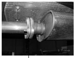
1.) REMOVE STOCK **EXHAUST BY UNCLAMPING** AT THE FLANGE LOCATED **JUST BEHIND THE CATALYTIC CONVERTER.** NEXT, CUT THE TAILPIPE OFF JUST BEHIND THE MUFFLER AND THEN REMOVE THE MUFFLER. REMOVE ALL HANGERS FROM RUBBER GROMMETS, LEAVE GROMMET IN PLACE. USE WD-40 FOR EASIER REMOVAL, NEXT REMOVE REAR CLAMP AND YOU CAN NOW REMOVE THE TATI PTPF.
