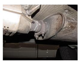
TO REMOVE STOCK EXHAUST UN-CLAMP IT FROM THE CLAMP LOCATED JUST **BEHIND THE CATALYTIC** CONVERTER. YOU MAY NEED TO HEAT THE CLAMP UP FOR EASIER REMOVAL. ALSO YOU MAY **NEED TO UN-BOLT** THE REAR TAILPIPE HANGER TO MAKE IT EASIER TO REMOVE STOCK **EXHAUST AND INSTALL NEW** EXHAUST.
