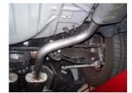
6. Install passenger side tailpipe/muffler assembly #C. Insert all welded hangers into rubber grommets. Secure tailpipe with clamp #D. Do not tighten.
