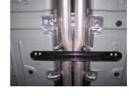
7. Now go back and make sure the first two mufflers in the middle are level. Then push up on factory cross member before tightening clamps. Then tighten X pipe. Next, with both tailpipes in place tighten all bolts and clamps securely.
