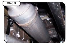
Install muffler #B onto head pipe #A 1 1/2"-2" with the louvers facing towards the converter. Use a jack stand to support the muffler. Use clamp #E to secure the muffler to the headpipe. Do not tighten. Muffler inlet is looking into the louvers. Outlet should be at the 10' O'clock position.
