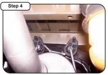
Next, install band clamp # F onto muffler, attaching with bolt kit #G. Insert hangers into rubber grommets. Do not tighten.
