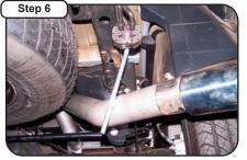
Attach Stainless Steel Tip. When you have everything in place, firmly tighten all bolts and clamps down securely. Use stainless steel cleaner and a Scotch Brite pad weekly to prevent tip from discoloration. Inspect all fasteners after 25-50 miles of operation and re-tighten if necessary.
