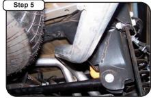
Install tail pipe #C into muffler 1 1/2" to 2". Use clamp #E to secure. Do not tighten. Insert welded hangers into rubber grommets.
