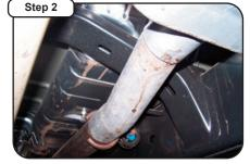
Install head pipe # A onto your existing stock front pipe and attach with clamp #E. Do not tighten . Insert welded hanger into rubber grommet.
