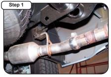
To remove the stock exhaust, remove your factory exit pipes. Next, remove your tailpipe by unbolting from the back of your stock muffler. Remove your factory muffler from the clamp in front of it. Use WD-40 to aid in removal of facotry grommet that will be re-used.
