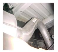
Install the over axle tailpipe # C into the muffler 1-1/2" to 2". Secure to the muffler using clamp # F. Do not tighten.
