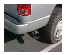
Install stainless steel tip. Clamp down. When you have everything in place, firmly tighten all bolts and clamp down securely. To clean stainless steel tip use any stainless steel cleaner.
