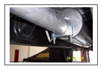
Install muffler #B onto head pipe # 1-1/2" to 2" with the louvers facing towards the converter. Use a jack stand to support the muffler. Use clamp #F to secure the muffler to the head pipe. Do not tighten. Muffler inlet is looking into the louvers.
