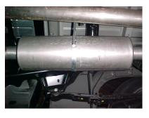
INSTALL MUFFLER #B ONTO HEADPIPE #A 1-1/2" TO 2" WITH THE LOUVERS FACING TOWARDS THE CONVERTER. USE A JACK STAND TO SUPPORT THE MUFFLER. USE CLAMP #F TO SECURE THE MUFFLER TO THE HEADPIPE. DO NOT TIGHTEN. MUFFLER INLET IS LOOKING INTO THE LOUVERS.
