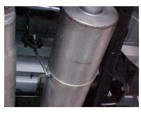
SLIDE BAND CLAMP #G ONTO MUFFLER #B. INSERT HANGERS INTO RUBBER GROMMETS.
