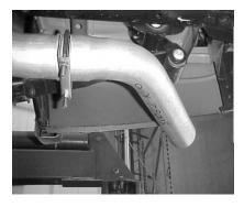
NEXT CONNECT THE TURN OUT PIPE #C TO THE OVERAXLE PIPE USING CLAMP #E. DO NOT TIGHTEN.
