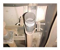
UNCLAMP EXHAUST IN FRONT OF STOCK MUFFLER. IF YOU HAVE AN EXTENSION PIPE BETWEEN THE CONVERTER AND MUFFLER- DO NOT REMOVE! LEAVE ALL RUBBER GROMMETS IN PLACE. INSTALL HANGERS AS PROVIDED.
