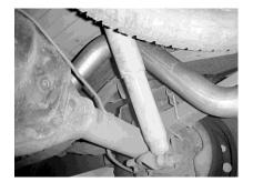
Install rear extension pipe #B and connect to muffler using clamp #F. Install over-axle tailpipe #C to extension pipe and attach using clamp #F.
