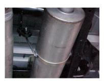
SLIDE BAND CLAMP #G ONTO MUFFLER WITH BOLT KIT # H. INSERT HANGERS INTO RUBBER GROMMETS.
