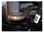
4. Install headpipe #A onto vour existing stock front pipe and secure with clamp #F. Do not tighten.
