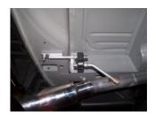
8. Install driver side over axle tailpipe #D into the muffler 1.5-2". Use clamp #G to secure. Do not tighten. Insert welded hanger into rubber grommet.
