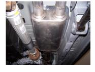
9. Install stainless steel tips. Clamp down. When you have everything in place, firmly tighten all bolts and clamps down securely. Use stainless steel cleaner and a Scotch Brite pad weekly to prevent tip from discoloration. Inspect all fasteners after 25-50 miles of operation and re-tighten as necessary.
