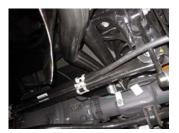
6. Install tailpipe #c into muffler 1.5-2". Insert welded hangers into rubber grommets use clamp #e to secure together. Do not tighten
