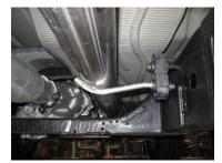
your existing stock flange and secure using the stock hardware. Do not tighten. Insert welded hanger into rubber grommet.
