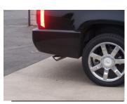
7. Install stainless steel tip #E. Clamp down. When you have everything in place, firmly tighten all bolts and clamps down securely. Use stainless steel cleaner and a Scotch Brite pad weekly to prevent tip from discoloration.
