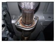
2. Remove the stock exhaust by removing it from the 2-bolt flange located in front of the muffler. Disengage the welded hangers using WD-40 from the OEM rubber grommets. Do not damage stock nuts and bolts or remove the rubber grommets as you will reuse them to mount your new system. Now, cut off tailpipe and remove exhaust.
