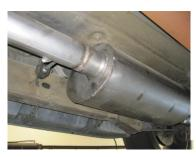
**4.** Install muffler #B onto head pipe 1½"-2" with the louvers facing towards the converter. Use a jack stand to support the muffler. Use clamp #F to secure the muffler to the headpipe. DO NOT TIGHTEN. Muffler inlet is looking into louvers.
