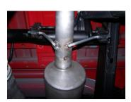
4. Slide the muffler #B into the headpipe at least 1.5"-2". Use a jack stand to support the muffler. Use clamp #E to secure muffler assembly to the headpipe. The outlet of the muffler will be at approximately 11 o'clock. The muffler inlet is looking into the louvers. Do not tighten.
