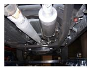
4. Install muffler #B onto headpipe 11/2"-2" with the louvers facing towards the converter. Use a jack stand to support the muffler. Use clamp #F to secure the muffler to the headpipe. Do not tighten. Muffler inlet is looking into the louvers.
