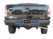
8. Install stainless steel tip #E. Clamp down. When you have everything in place, firmly tighten all bolts and clamps down securely. Use stainless steel or aluminum cleaner to polish tips. Inspect all fasteners after 25-50 miles of operation and re-tighten as necessary.
