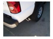
**7.** Install stainless steel tip #E. Clamp down. When you have everything in place, firmly tighten all bolts and clamps down securely. Use stainless steel cleaner and a Scotch Brite pad weekly to prevent tip from discoloration. Inspect all fasteners after 25-50 miles of operation and re-tighten as necessary.
