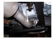
**3.** Install headpipe #A onto your exisiting 2-bolt flange reuse your factory nuts to secure. Do not tighten. Insert welded hanger onto rubber grommets.
