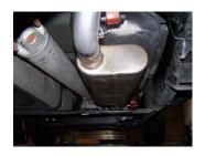
**4.** Install muffler onto head pipe #A. 11/2"-2" with the louvers facing towards the converter. Use a jack stand to support the muffler. Use clamp #E to secure the muffler to the headpipe. DO NOT TIGHTEN. Muffler inlet is looking into the louvers. Outlet will be on the drivers side.
