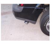
**9.** Install stainless steel tip #D. Clamp down. When you have everything in place, firmly tighten all bolts and clamps down securely. Use stainless steel cleaner and a Scotch Brite pad weekly to prevent tip from discoloration. Inspect all fasteners after 25-50 miles of operation and Re-tighten as necessary.
