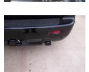
**11.** Install stainless steel tips. Clamp down. When you have everything in place, firmly tighten all bolts and clamps down securely. Use stainless steel cleaner and a Scotch Brite pad weekly to prevent tip from discoloration. Inspect all fasteners after 25-50
