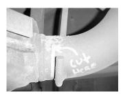
LAY OUT THE EXHAUST ON THE FLOOR SO IT LOOKS LIKE THE DRAWING AND COMPARE PARTS TO THE MANUAL. TO REMOVE THE STOCK **EXHAUST CUT YOUR** TAILPIPE OFF JUST BEHIND THE FACTORY HANGER, NEXT MEASURE 34" IN FRONT OF YOUR CONVERTER AND CUT, THEN UNCLAMP IT FROM THE CLAMP IN FRONT OF THE MUFFLER. THEN REMOVE THE STOCK MUFFLER AND EXTENTION PIPE. LEAVE ALL RUBBER GROMMETS IN PLACE, USE WD-40 TO AID IN REMOVAL OF HANGERS.
