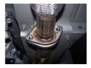
2. To remove the stock exhaust, unbolt it at the 2-bolt flange located in front of the muffler. Disengage the welded hangers using WD-40 from the OEM rubber grommets. Do not damage stock nuts and bolts or remove the rubber grommets as you will re-use them to mount your new system. Now, cut off tailpipe and remove exhaust.
