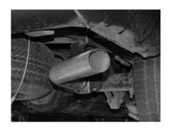
INSTALL OVERAXLE TAILPIPE #C INTO MUFFLER 1-1/2" TO 2" USING CLAMP #F TO SECURE THE TAILPIPE TO THE MUFFLER. DO NOT TIGHTEN. INSTALL TURNOUT PIPE #D ONTO TAILPIPE. INSTALL TAILPIPE HANGER #I INTO RUBBER GROMMET AND ATTACH IT TO THE TAILPIPE. DO NOT TIGHTEN. NOW TIGHTEN ALL CLAMPS, BOLTS AND FLANGE
