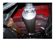
4. Install muffler #B onto headpipe #A 1.5-2" with louvers facing towards the converter. Use a jack stand to support the muffler. Outlet of muffler will be at 12 o'clock position.
