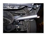
7. Install exit pipe #H onto the tailpipe, use clamp #F to secure the two pipes together. (Rotate for the best fit on your vehicle.)
