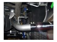
**6.** Use clamp #E to secure tailpipe to the muffler. DO NOT TIGHTEN.
