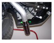
7. Install stainless steel tip. Clamp down.
