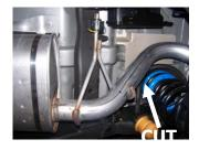
**2.** To remove the stock exhaust, remove it from the two bolt flange in front of the muffler. Do not disgard you will re-use bolts. Disengage the welded hangers using WD-40 from the OEM rubber grommets. Do not damage or remove the rubber grommets as you will reuse them to mount your new system. Now, cut off tailpipe before and after rear axle for removal.
