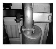
INSTALL MUFFLER WITH THE INSIDE LOUVERS FACING FORWARD TOWARDS THE CONVERTER. USE CLAMP #E AT THE INLET OF THE MUFFLER. DO NOT TIGHTEN. MUFFLER OUTLET WILL BE POSITIONED AT ABOUT 8 - 9 O'CLOCK. THE MUFFLER INLET IS LOOKING INTO THE LOUVERS.
