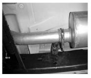
BOLT HEADPIPE #A RE-USING THE FACTORY NUTS. DO NOT TIGHTEN. INSTALL HANGER #G ONTO HEAD PIPE. SLIDE HANGER INTO RUBBER GROMMENT.
