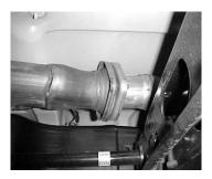
FOR AN EASIER REMOVAL OF THE FACTORY EXHAUST CUT THE TAILPIPE BEHIND THE REAR MUFFLER HANGER. THEN UNBOLT THE FLANGE BEHIND THE CONVERTER. KEEP THE BOLTS FOR YOU WILL REUSE THEM. USE WD-40 ON ALL HANGERS. LEAVE ALL FACTORY RUBBER GROMMETS IN PLACE.
