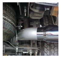
SLIDE EXIT PIPE # E ONTO OVERAXLE TAILPIPE INSERT WELDED HANGER INTO RUBBER GROMMET. USE CLAMP # I TO SECURE PIPES TOGETHER. DO NOT TIGHTEN. ROTATE PIPE UNTIL LEVEL.
