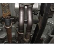
TO REMOVE STOCK EXHAUST, CUT 13" FROM THE FRONT OF THE MUFFLER, MEASURE TOWARDS THE FRONT OF THE VEHICLE. LEAVE ALL RUBBER GROMMETS ON THE HANGER. USE WD-40 TO AID IN THE REMOVAL OF EXHAUST AND HANGERS. SUPPORT THE CATALITIC CONVERTER BEFORE CUTTING.
