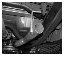
BOLT HEADPIPE #A TO THE STOCK FLANGE RE-USING THE FACTORY NUTS & BOLTS. INSERT WELDED HANGER INTO RUBBER GROMMET. DO NOT TIGHTEN.
