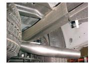
Install over axle tailpipe #C into muffler  $1\frac{1}{2}$ " to 2". Secure together with clamp #C. Do not tighten. Insert hanger into rubber grommet.
