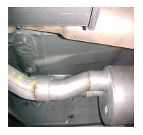
INSTALL HEADPIPE # A SLIP IT ONTO STOCK HEADPIPE USING CLAMP # H TO SECURE IT. DO NOT TIGHTEN. INSTALL HEADPIPE # B, SLIP IT ONTO THE STOCK HEADPIPE USING CLAMP # H TO SECURE THE HEADPIPE TO THE STOCK PIPE. DO NOT TIGHTEN.
