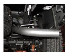
SLIDE TAILPIPE #D INTO MUFFLER 1-1/2" TO 2". INSERT WELDED HANGER INTO RUBBER GROMMET AND CLAMP DOWN TO REAR MUFFLER HANGER.
