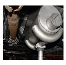
NEXT INSTALL MUFFLER #C. SLIDE IT ONTO HEADPIPE 1-1/2" TO 2". AND ATTACH USING CLAMPS # F. INLET OF MUFFLER SHOULD FACE TOWARDS THE MOTOR. MUFFLER INLET IS LOOKING INTO THE LOUVERS.
